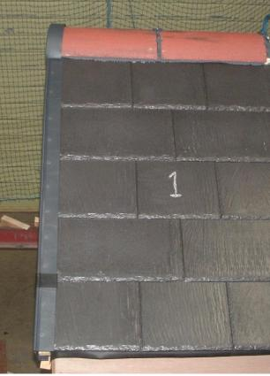
The testing showed that when installed as described in the manufacturers instructions, the Manthorpe SmartVerge<sup>®</sup> Linear Dry Verge System is capable of withstanding wind speeds of up to at least 48.5m/s (108mph). At this wind speed the verges showed no visible signs of distress and at the end of the testing there were no indications that the verges or their fixings had sustained any wind-induced damage.
