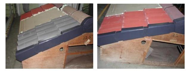
The testing showed that when installed as described in the manufacturers instructions, the Manthorpe Dry Verge System is capable of withstanding wind speeds of up to at least 48m/s. At this wind speed the verges showed no visible signs of distress and at the end of the testing there were no indications that the verges or their fixings had sustained any wind-induced damage.
