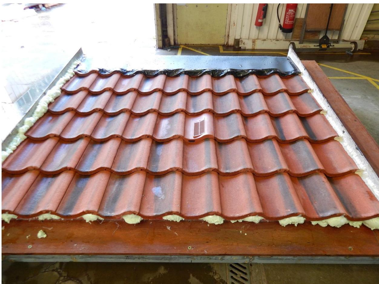
Figure 1 Single Pan Tile Vent installed with Redland Fenland tiles
