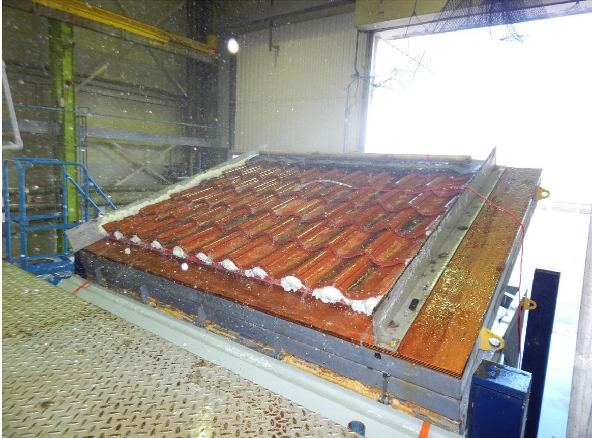
Figure 2 Manthorpe Single Pan Tile Vent with Redland Fenland tiles under test
