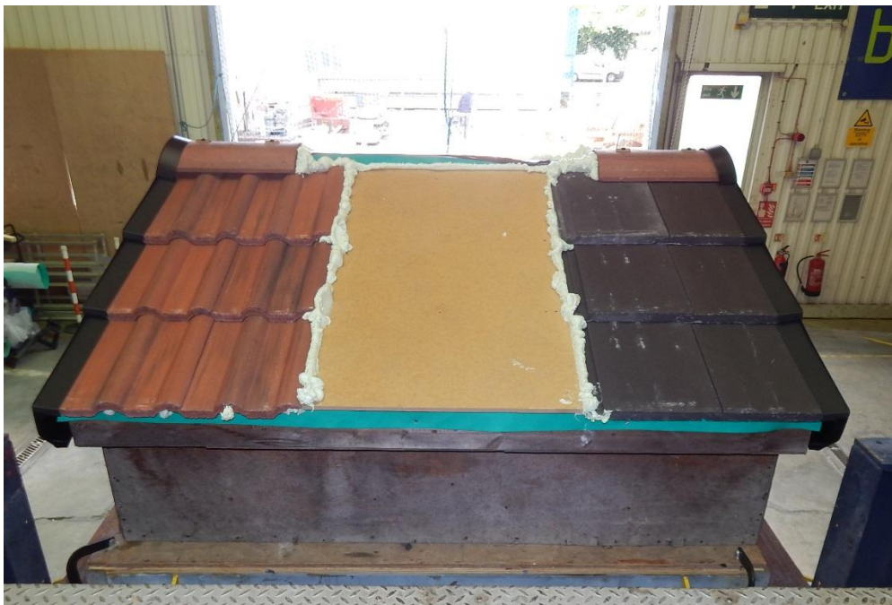
Figure 2 Manthorpe SmartVerge Polypropylene installed with flat and profiled tiles.
