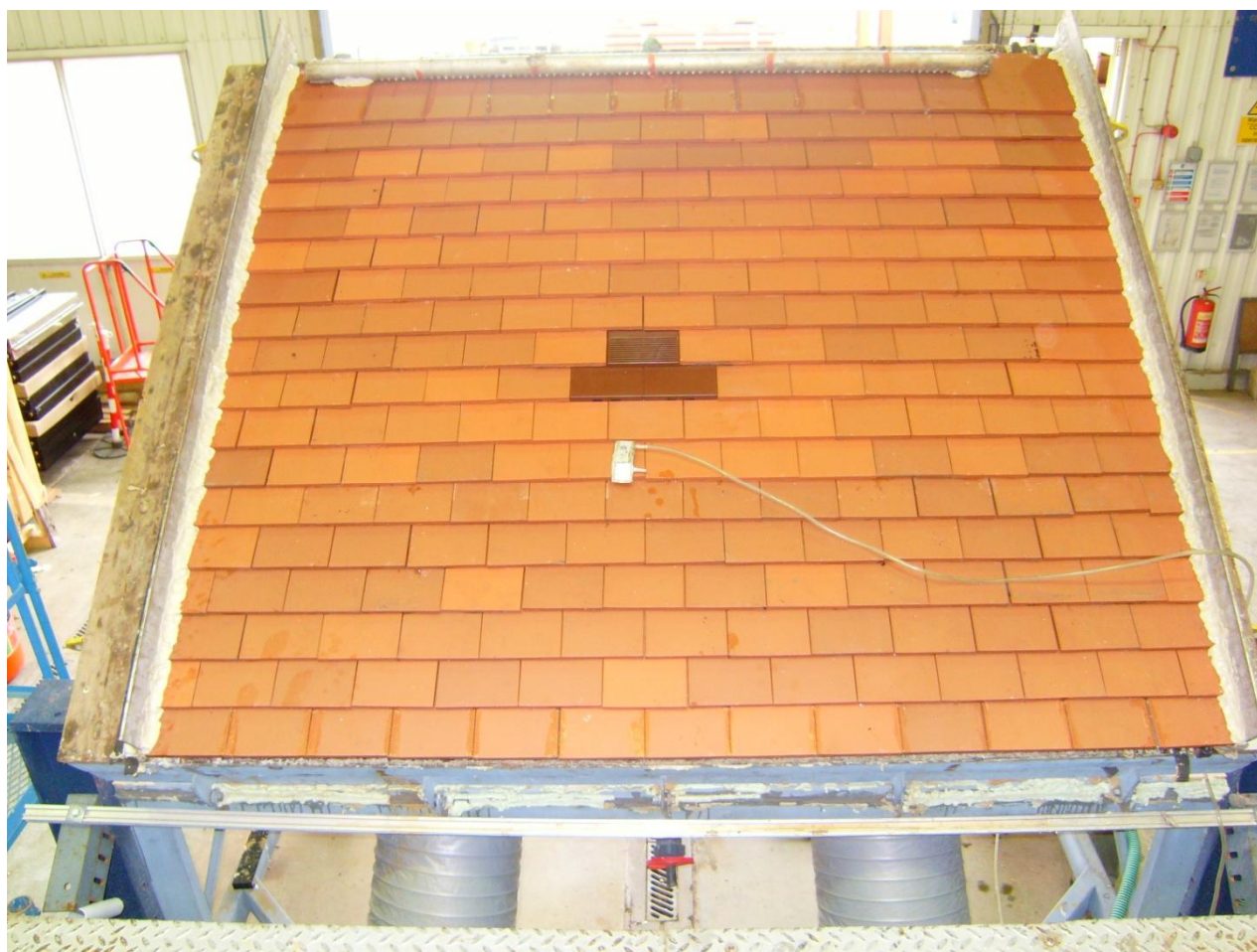
Figure 1 Manthorpe plain tile roof vent with Redland Rosemary plain clay tiles installed on the BRE driving rain test rig
