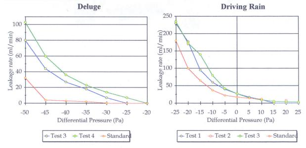
This illustrates just how well the vent tile has performed - the curve leaving the asymptote at -70Pa and -33Pa respectively. Subsequently a quick wind-driven rain test under the same conditions as the above graphs gave a leakage of 83ml/min for the vent alone at a differential pressure of -75Pa. The graphs above, however, are for a 1m² area of tiles.
