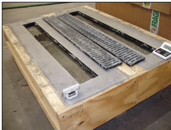
Figure 3: Photograph showing 2 of the 3 assemblies for watertightness test of channel body
