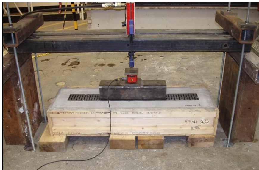
Figure 4: Photograph showing assembly for load test of SmartDrain unit
