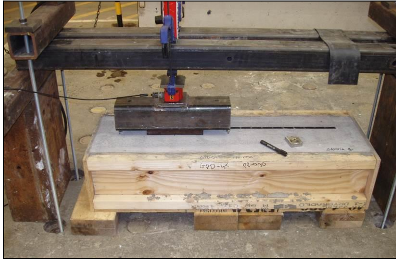
Figure 5: Photograph showing assembly for permanent set test of SlotDrain unit
