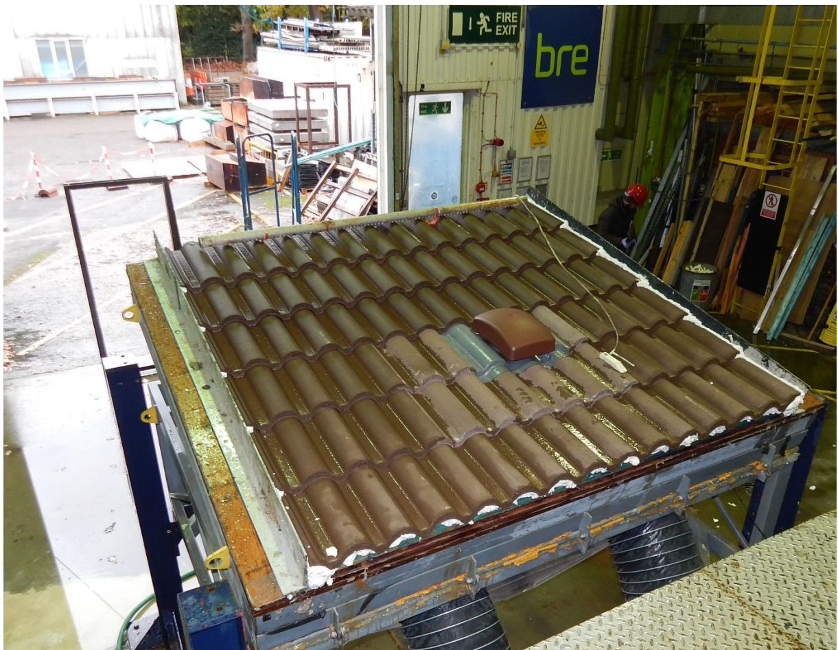
Figure 2 View of the Manthorpe Cowled Universal Roof Vent with a Large Format Bold Roll Tile installed on the BRE test rig
