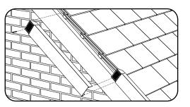
**5.** Continue on up the run of the verge, clipping and fixing each Linear Verge Unit consecutively at the toe and head to ensure a secure fit.
