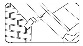
**6.** For roofs where the bottom course of tiles are tilted upwards, cover the nail head and joint using a **Verge Union**.
