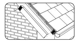
*4.* Hook the Linear Verge Unit over the top of the Fixing Clip and press firmly until it engages.
