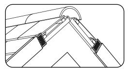
7. Continue to fit full lengths of the linear units up the run of the verge until all tiles have been covered or no full legnths can be fitted as shown.
