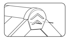
**9.** Align the Ridge End Cap with the top two verges and flex it over the units and the top of the ridge tile.
