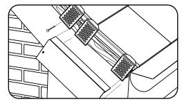
2. For roofs with a change in pitch at the eaves, use three fixing clips as shown. Saw a length of the Linear Verge Unit down to cover the full length of the tilted section of the verge. Hook the shortened Linear Verge Unit section over the top of both Fixing Clips and then push it on to the verge until it engages with both clips.
