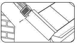
**3.** To prevent the shortened Linear Verge Unit from sliding down the verge, drill and fix the unit **10mm** from the edge into the batten as shown above.
