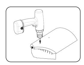
7. Fix the tile to the roof through hole (B), using the screw found in the Manthorpe GDRH roll-out hip kit or a suitable fixing.
