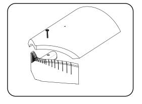
5. Push the product tight up against the underside of the tile ensuring that all of the tabs conform to the tile profile.
