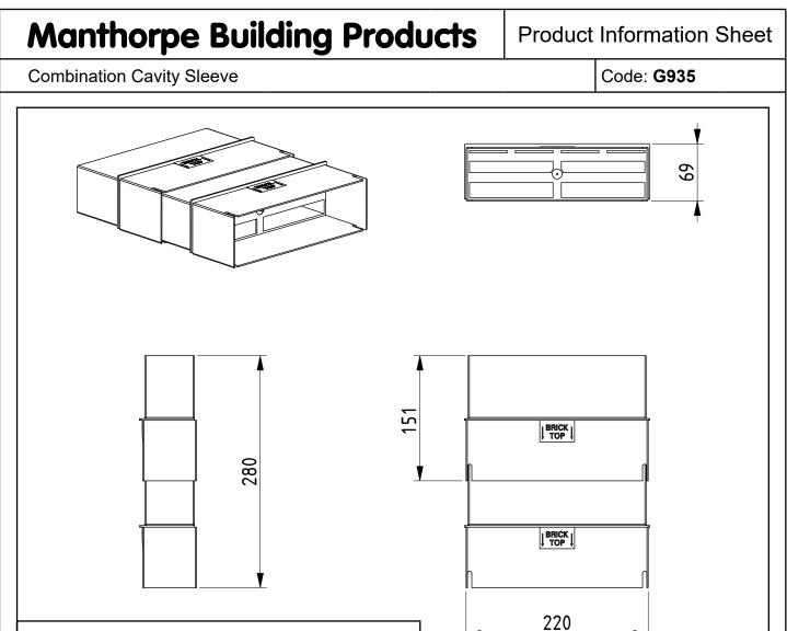
Each G935 assembly consists of 2 identical parts
