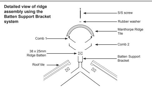
*NOTE:* This product should not be installed within close proximity to potentially hot elements of the roof structure, such as chimney pots or flue outlets, or on a roof surface which could reach excessively high temperatures, such as metal clad or glazed roofs.
