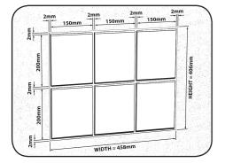
1. Calculate the total height and width of the access panel opening by measuring all tiles including separating and surrounding grout joints.
