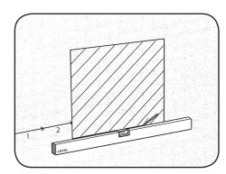
2. Mark out the opening, making sure it is square and level with a spirit level. (It may be worth calculating the distance of the opening from the outer edge of the wall and floor to avoid the need for cutting tiles when you come to tiling the perimeter of the wall).
