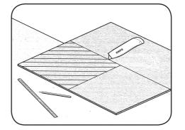
7. Using a suitable 6mm thick, water resistant tile backing board, mark out a panel 25mm smaller in both height and width than the wall opening.
