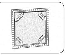
9. Insert the panel into the frame by engaging both hinges and then pushing the magnets together.
