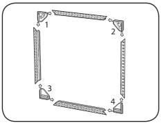
4. Assemble the frame with corner parts 1, 2, 3 and 4 as shown by sliding the 'T' section of the corner clips into the 'C' section of the extrusion.
