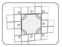
**10.** Using standard tiling practices, tile the wall outside of the frame.
