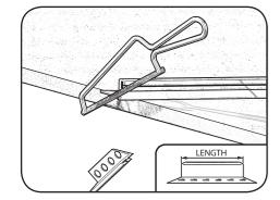
**3.** Saw four lengths of extrusion at 45° using a mitre saw or suitable hand saw to form a frame, equal in size to your openina.
