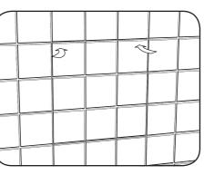
**11.** Tile the front of the panel leaving a thin gap between the outer tiles and the frame to allow the panel to open.
