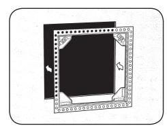
6. Push the assembled frame firmly into the wall opening so that the perforated flange sits tightly against the wall.
