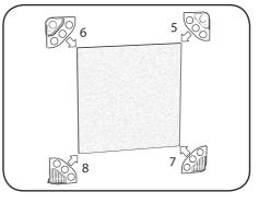
8. Attach the plastic corner parts 5, 6, 7 and 8 to the backing board as shown so that they sit firmly against the edges of the board.
