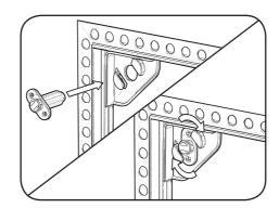
5. Assemble both magnetic touch latches to the frame by inserting them into corner parts 1 and 2 as shown then twisting 90° clockwise until both latches "click" into place.
