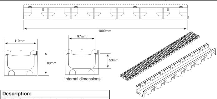
The Manthorpe 1m linear drainage channel is an easy and effective way of removing unwanted standing water into a domestic drain. The channel and grate have been independently load tested and gained an A15 load rating in accordance with BS EN 1433:2002. (BRE Test Report 289 099)
