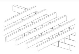
1. Lay out joists to ensure they are the correct length. There should be at least 90mm bearing on the block
