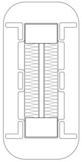
If using Timber engineer Joists, tightly pack gaps around webs with mineral wool to maintain the thermal and fire protection properties of the wall. This is of particular importance in party walls.
