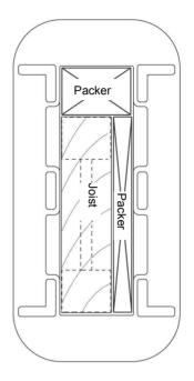
If using joists smaller than the joist seal the gaps around the joist should be filled to prevent movement and maintain the structural integrity of the wall and floor.
