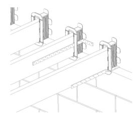
3. Restraining straps should be fitted at 2m centres to comply with building regulations. Trim out one of the pockets in the appropriate position using a sharp knife, push the strap through the joist seal and secure to the ioist.
