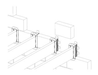
**4**. To fill in between the joists use cut blockwork. Mortar each block into position. Take care not to damage the foam seal on the inner flange.
