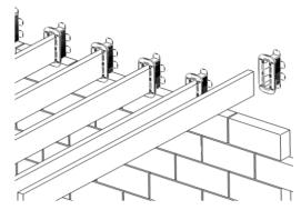
2. Push joist seal on to the end of each joist and place back on the blockwork. Pack joist level if required.
