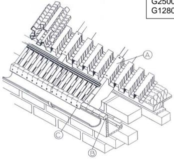
rolled out over the full length of the eaves and pulled to adjust to the correct roof truss centres then nailed or stapled down to secure in position as shown.
