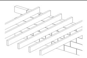
**1**. Lay out joists to ensure they are the correct length. There should be at least 90mm bearing on the block work.
