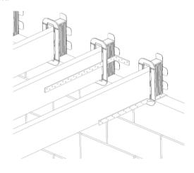
**3**. Restraining straps should be fitted at 2m centres to comply with building regulations. Trim out one of the pockets in the appropriate position using a sharp knife, push the strap through the joist seal and secure to the joist.
