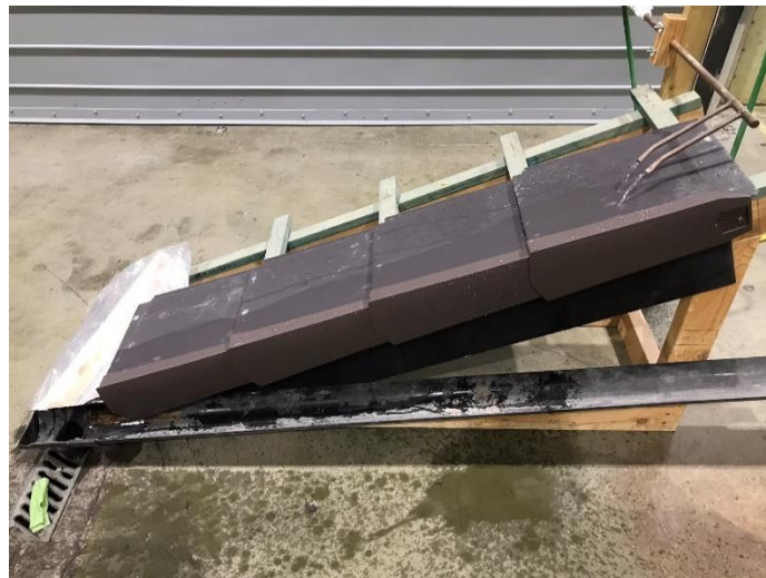
Figure 9: Manthorpe dry verge under the rain drainage test.
