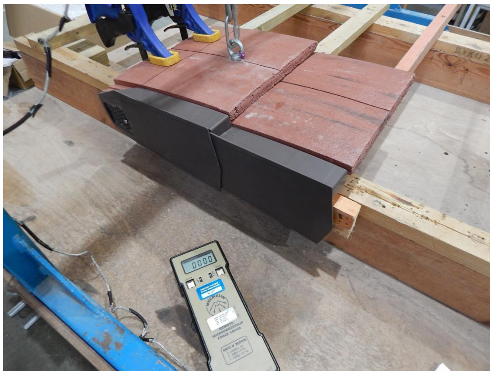
Figure 4. Manthorpe verge units prior to test.
