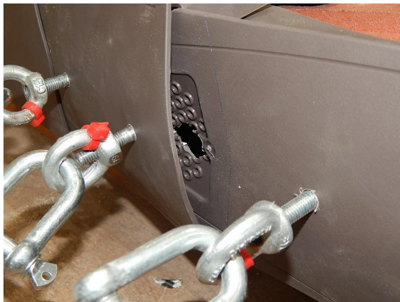
Figure 2. Ultimate failure of Manthorpe verge unit.
