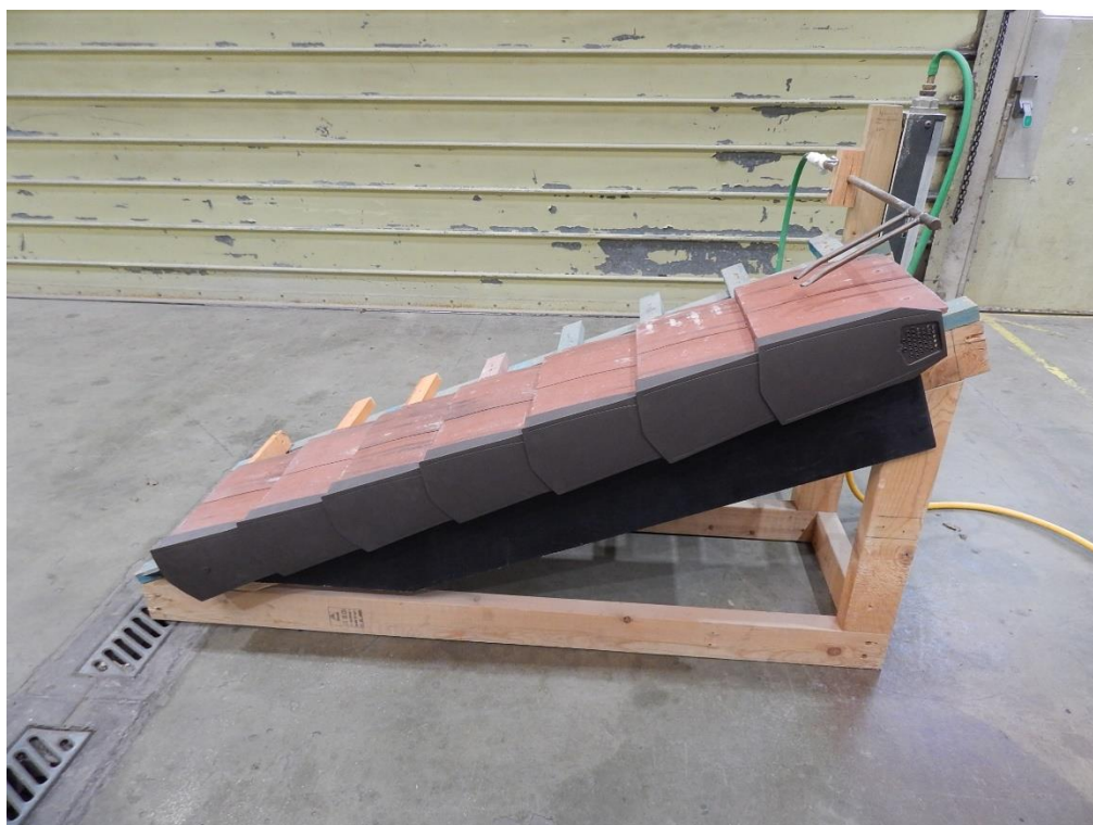
Figure 6. Manthorpe SmartVerge Interlocking Plain Tile Verge System prior to the rain drainage test.
