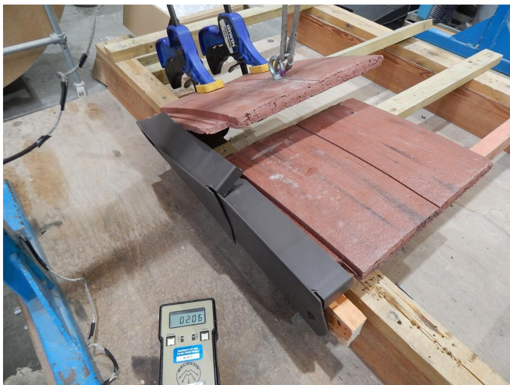
Figure 5. Image to highlight the ultimate failure of the Manthorpe verge.
