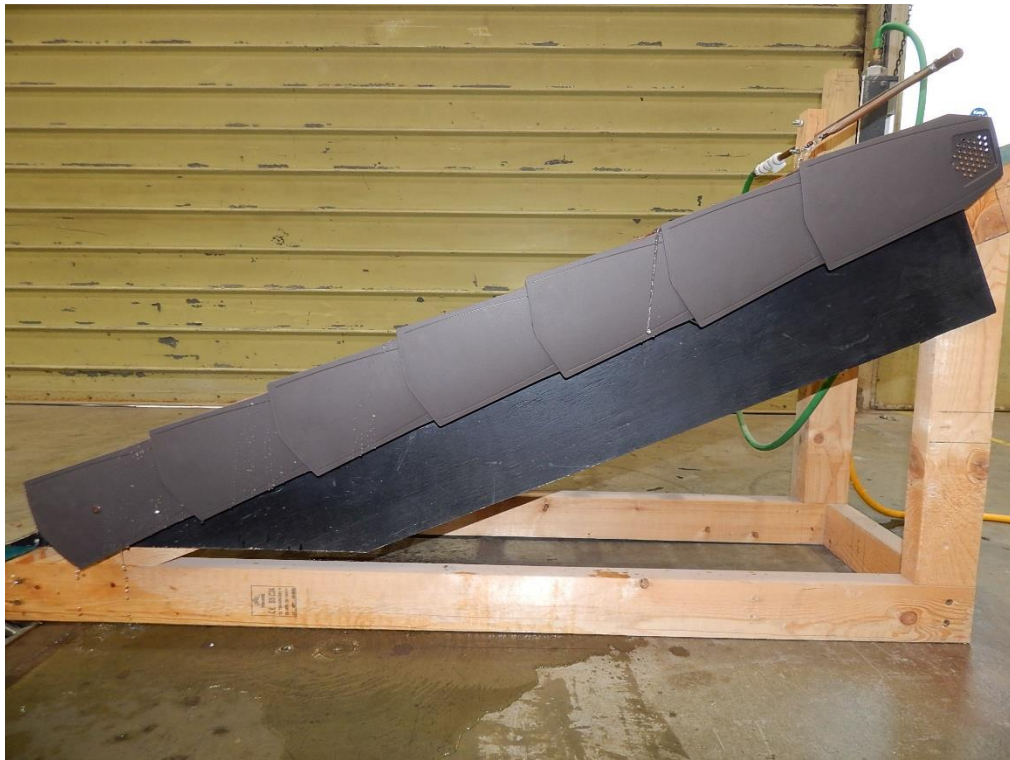
Figure 7. Stream of water on verge unit during rain drainage test.
