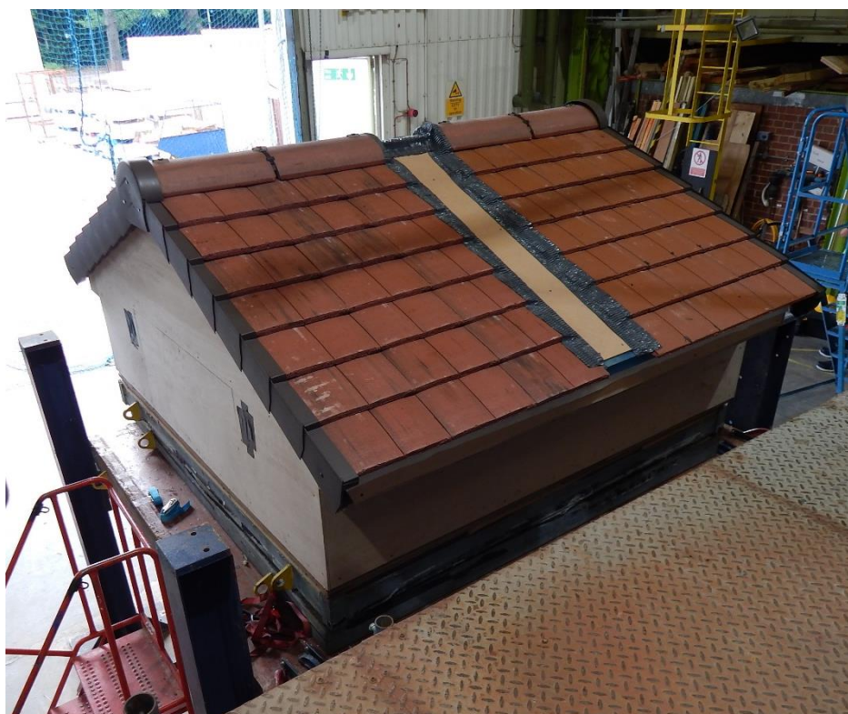
Figure 1. Manthorpe SmartVerge Interlocking Plain Tile Verge system installed with interlocking plain tiles.
