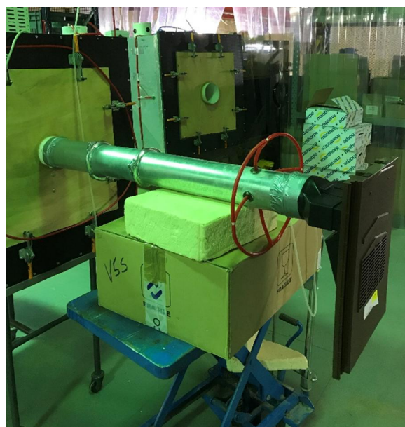
Figure 5 Ventilator terminal installed on test rig
