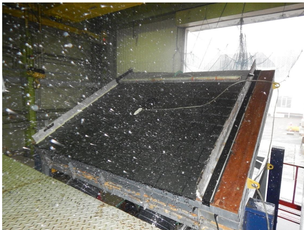
Figure 3 Manthorpe Small Format Vent Tile with Natural Slate tiles under test
