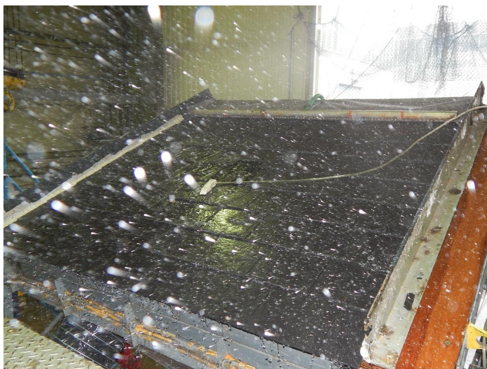
Figure 4 Manthorpe Small Format Vent Tile with Fibre Cement tiles under test
