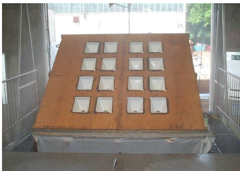
Figure B6 View of the 16 rainfall collection buckets on the test rig
