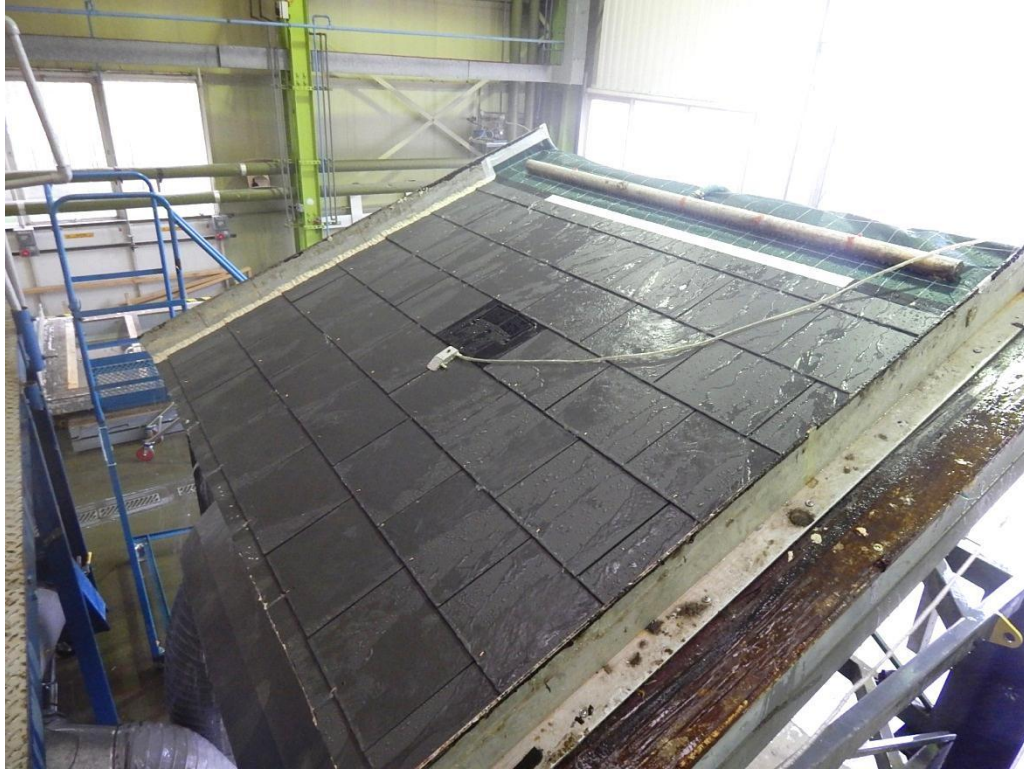
Figure 2 Manthorpe In-line slate vent with 600mm x 300mm fibre cement slates under test
