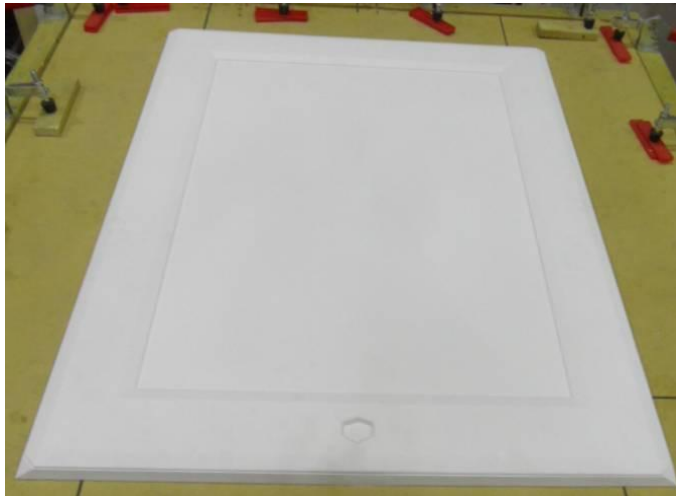
Figure 1 View of Manthorpe GL250 Loft Access Hatch before test.
